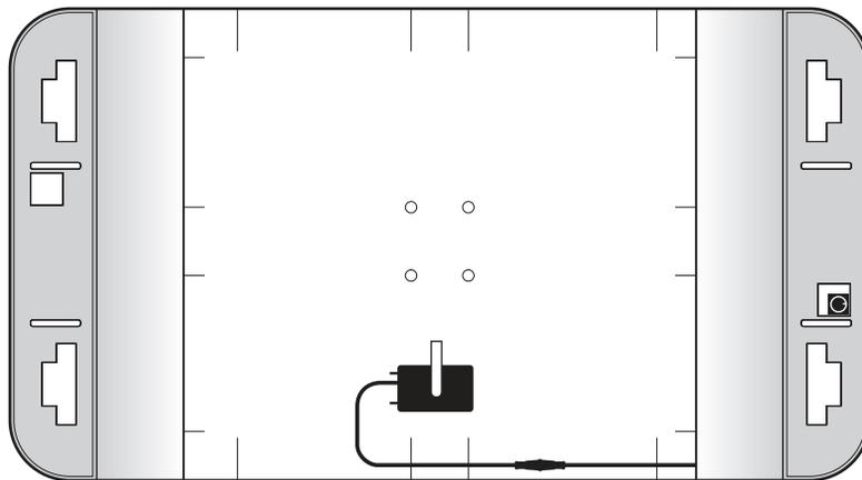
Anchor the pump on the bottom of the panel and adjust the pipe to point inwards.
